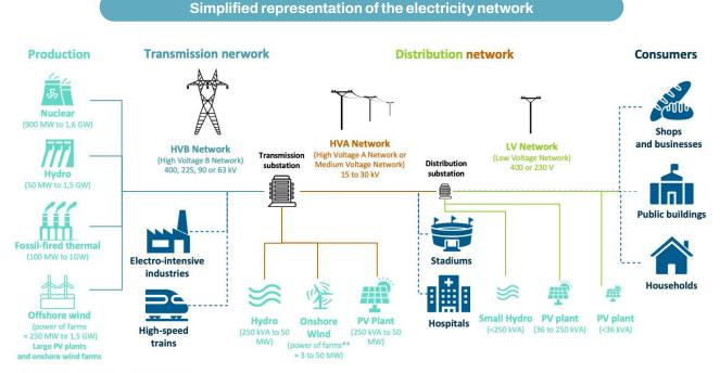
\* Unit capacity of an offshore wind : 6 to 15 MW \*\* Unit capacity of an offshore wind : 3 to 5 MW
